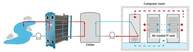
Or by free-cooling from a nearby lake, river or sea. Tranter's plate and frame heat exchangers can be constructed with plates in stainless steel, high alloy or titanium plate material for trouble-free operation, depending on the available cooling source.
