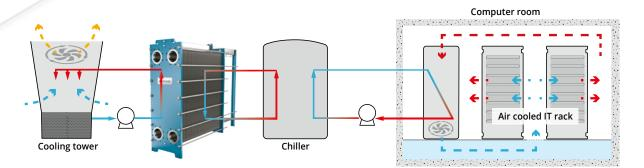
To make the datacenter more sustainable a Tranter plate and frame heat exchanger can be installed as a cooling tower intermediate cooler.
